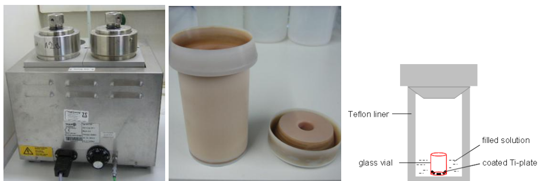
Figure 3.2 Images of autoclave pressure vessel and heating oven (left), Teflon liner (middle), and the schematic diagram (right) for solvothermal processing of electrode coatings.
