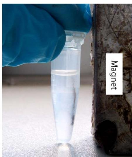
**Figure 37: Superparamagnetic  $\text{Fe}_3\text{O}_4$  NP containing Agarose microfibers ( $\varnothing = 5 \mu\text{m}$ ) in  $\text{H}_2\text{O}$  after template decomposition and phase transfer in presence of a magnet.**
