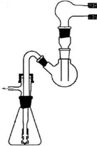
Figure 9: Schematic view of a twin-stage impinger which was used by Grainger et al. [165]
