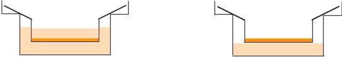
Figure 5: Liquid covered cultivation (left side) differs from the air-liquid interface cultivation (right side). LCC cells are covered with medium from both sides, whereas ALI cells are exposed to air at their apical side
