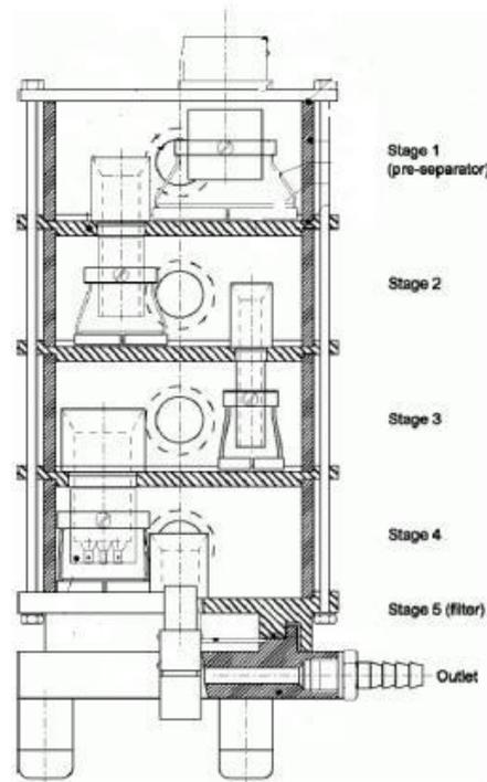
Figure 8: Schematic view of a multi-stage liquid impinger which was used by Bur et al. [164]
