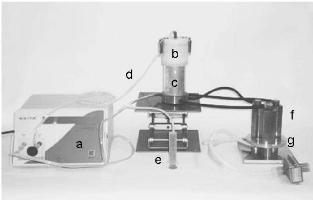
Figure 10: Schematic view of the PADDOCC system I: air flow control unit, II: aerosolisation unit, III: deposition unit, a: Akita<sup>®</sup> device, b: HandiHaler<sup>®</sup> chamber with capsule, c: aerosolisation chamber, d: aerosolisation tube, e: y-shaped tube with syringe, f: sedimentation chamber, g: sampling unit, h: sampling unit (with Snapwell<sup>®</sup>) in ventilation mode, i: sampling unit (with Snapwell<sup>®</sup>) in deposition mode
