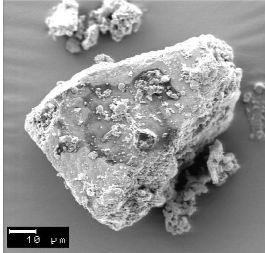
Figure 4: Typical dry powder formulation comprising of large carrier particle covered with small drug crystals
