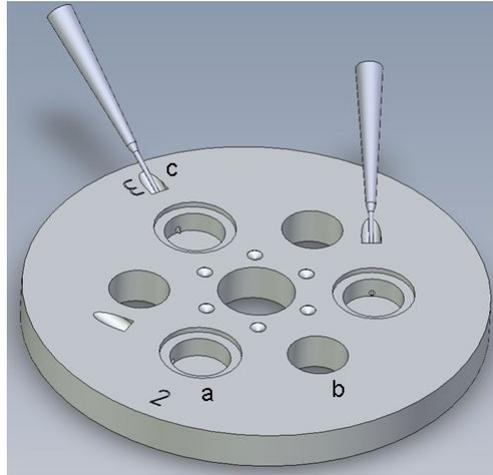
Figure 13: Sampling unit with alternately sampling wells (a) and ventilation holes (b) as well as pipetting ports for sample taking (c)
