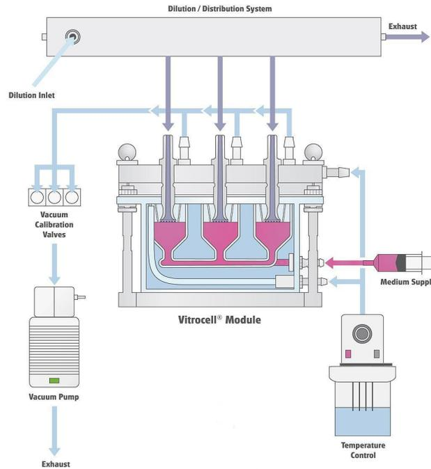
Figure 7: An overview of the CULTEX-Vitrocell system: the gas mixture is drawn to the three vessels which contain air-liquid interface cultured cell monolayer, viability of cells is ensured by medium supply and temperature control (modified according to [153], by courtesy of VITROCELL®)
