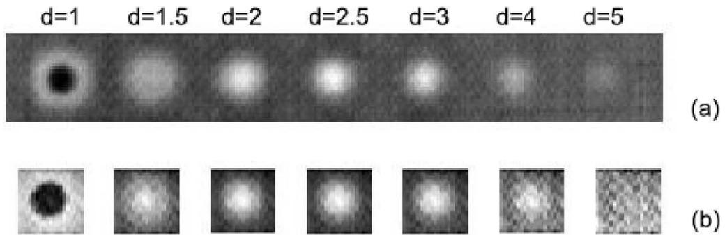
Figure 3.6: (a) Defect measurements for defects situated at different depths; (b) Simulations of the defects by taking  $\alpha = [0.5 \ 0.5 \ 0.28] \text{ mm}^2 \cdot \text{s}^{-1}$  at a lockin frequency of 0.01 Hz.
