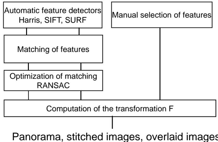
Figure 4.1: Scheme of the required steps to compute the transformation  $F$ . After features have been selected either manually or automatically, they have to be matched and the outliers have to be eliminated with the algorithm RANSAC.
