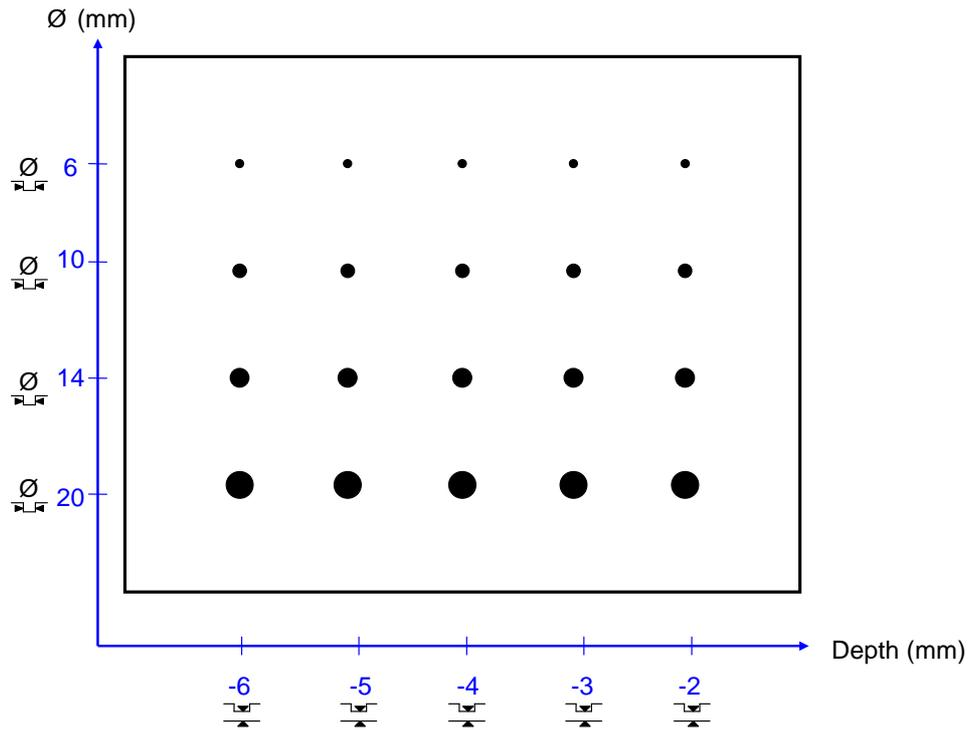
Figure 7.15: Scheme of the CFRP test-part with blind holes.
