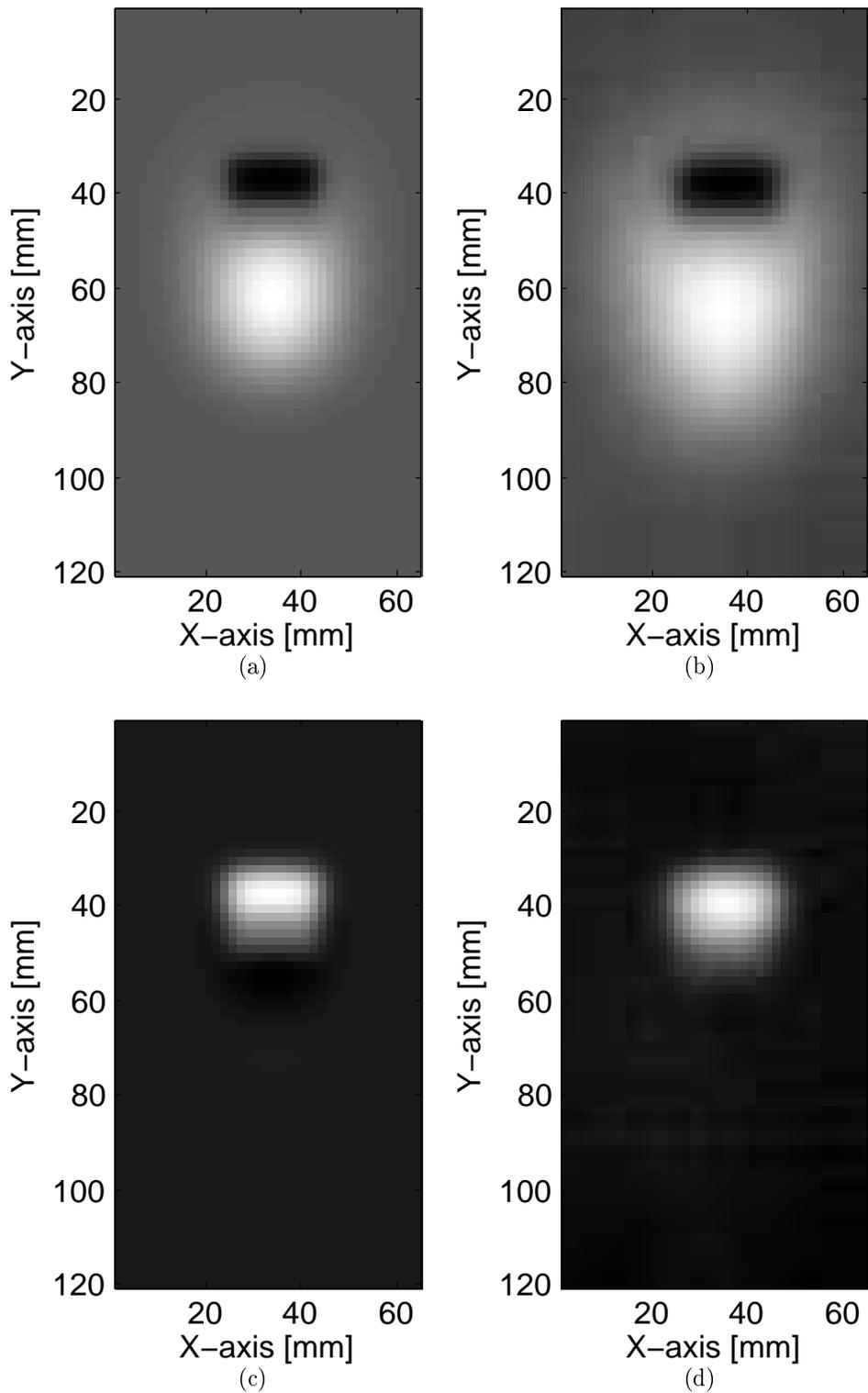
Figure 5.23: Simulations (left) and measurements (right) of the phase images of a wedge at frequencies (a-b) 0.005 Hz and (c-d) 0.05 Hz.
