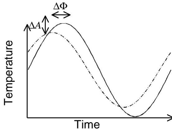
Figure 2.6: Computation of phase and amplitude images.
