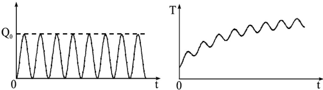
Figure 3.2: (a) Periodic heat modulation and (b) surface temperature vs. time in the non-stationary case [Wu96].
