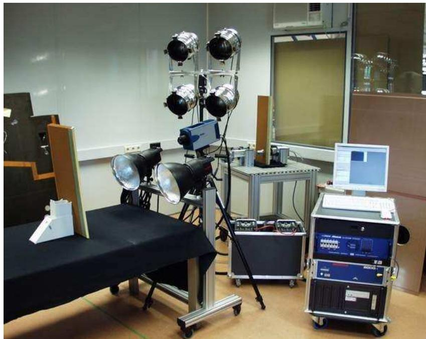
Figure 5.2: Thermography set-up of the Edevis company.
