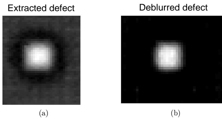
Figure 5.15: Deconvolved rectangular defect situated at 2 mm depth from the phase image at a frequency 0.03 Hz.
