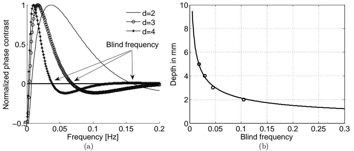
Figure 5.3: (a) Theoretical phase contrast function vs. frequency at different defect depths  $d$ , given here in mm; (b) Depth vs. the blind frequency (here  $\alpha_z = 0.22 \cdot 10^{-6} \text{ m}^2 \cdot \text{s}^{-1}$ ).
