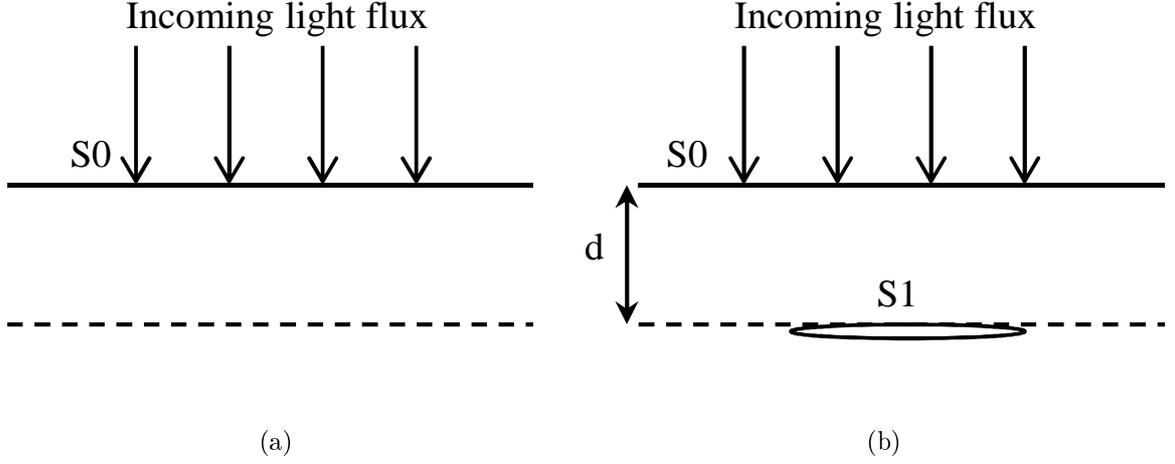
Figure 3.5: Scheme of the light flux on the semi-infinite part; (a) without a defect and (b) with a defect. The defect is represented by  $S_1$  and is at a depth  $d$ .
