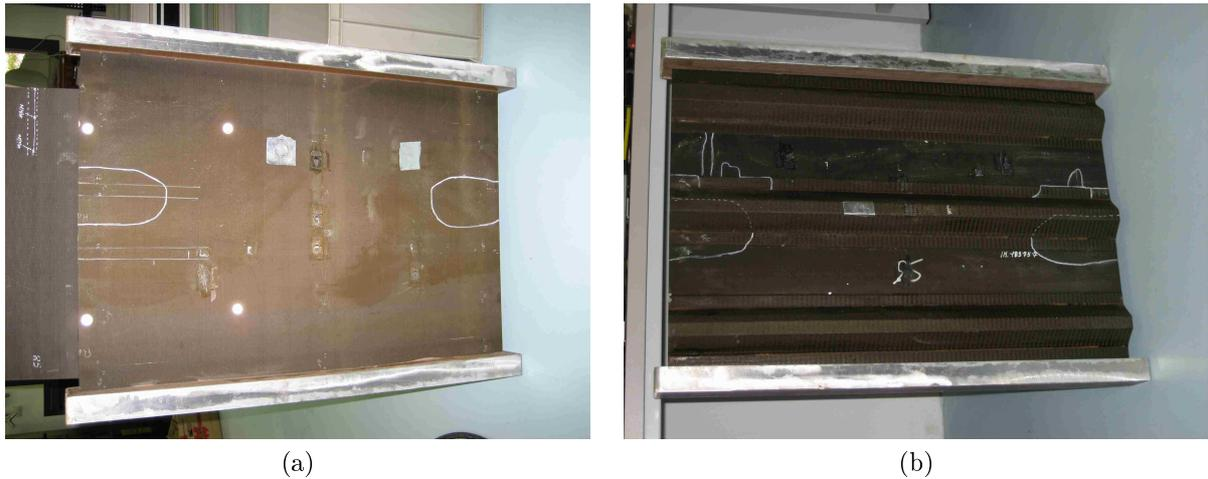
Figure 7.1: Image of the CFRP stiffened panel (a) from the front side (b) from the rear side (Component IV).
