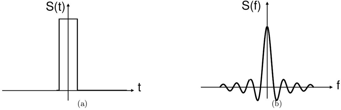
Figure 7.13: (a) Representation of a rectangle pulse excitation and (b) corresponding Fourier-transform.
