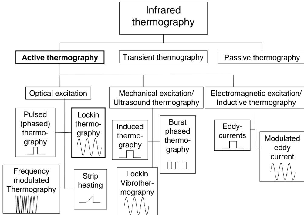
Figure 2.2: Overview of thermographic techniques.
