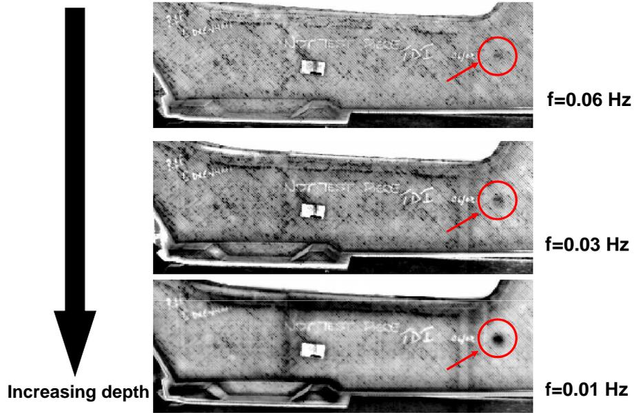
Figure 2.11: Example of lockin phase images of an impact damage in a CFRP component obtained at different frequencies.
