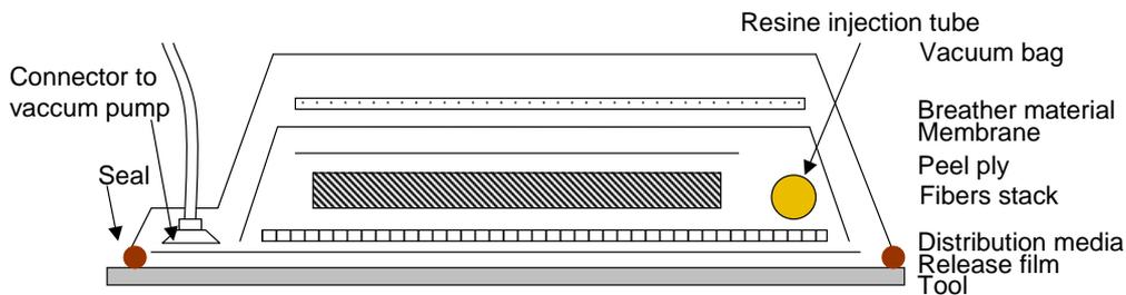
Figure 1.5: Layers of the set-up of a vacuum bag molding with dry fibers material.
