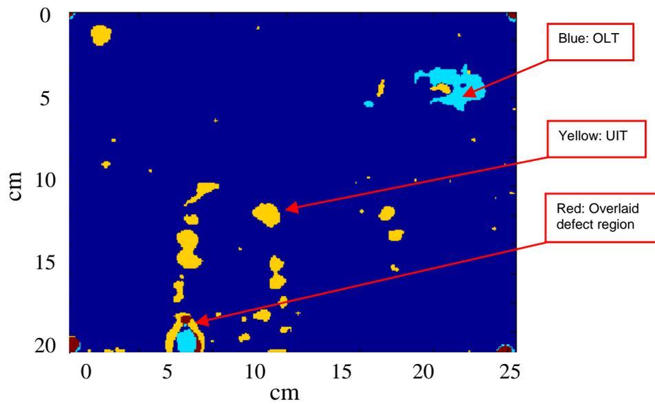
Figure 7.7: Overlay of segmented UIT and OLT images. The colored areas represent the defect region: blue being from the segmented OLT image, yellow being from the segmented UIT data, and red being the defect area detected in UIT and OLT.
