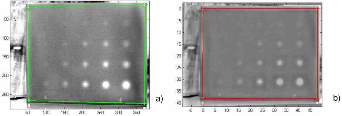
Figure 4.12: Equalization of images using photogrammetry; (a) Original image (OLT, phase image, 0.01 Hz); (b) rectified image with scale.
