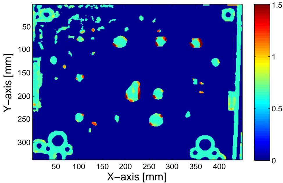
Figure 5.21: Depth-map obtained of the defects on an aircraft door. The color scale indicates the depth in mm.
