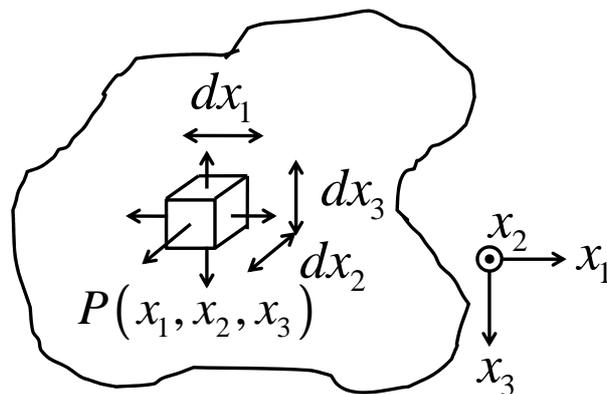
Figure 3.1: Flow of heat in a volume element.
