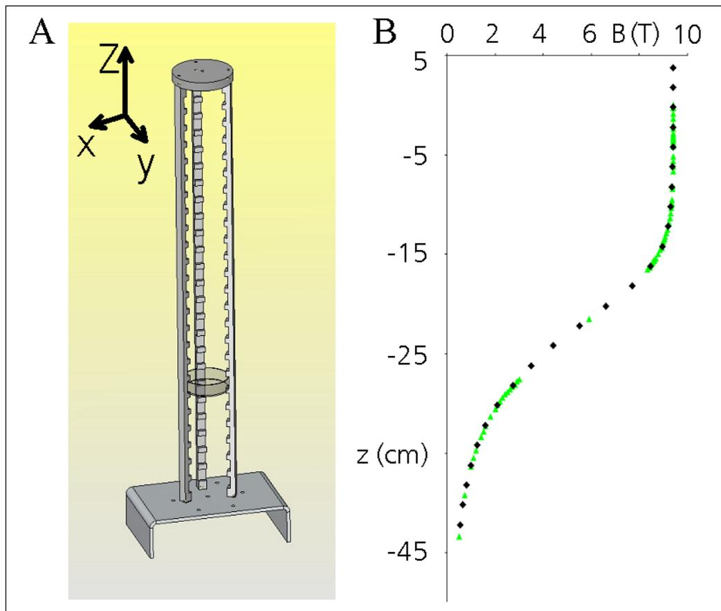
**Figure 3.1.:** Magnetic field exposure. (A) The rack in which the Petri dishes with the cells were positioned.  $z$  direction is the direction of the static magnetic field (courtesy of Martin Benecke). (B) Characterisation of the magnetic field. Green triangles represent measured field strengths, blue diamonds indicate the field strengths at the respective positions in the rack.
