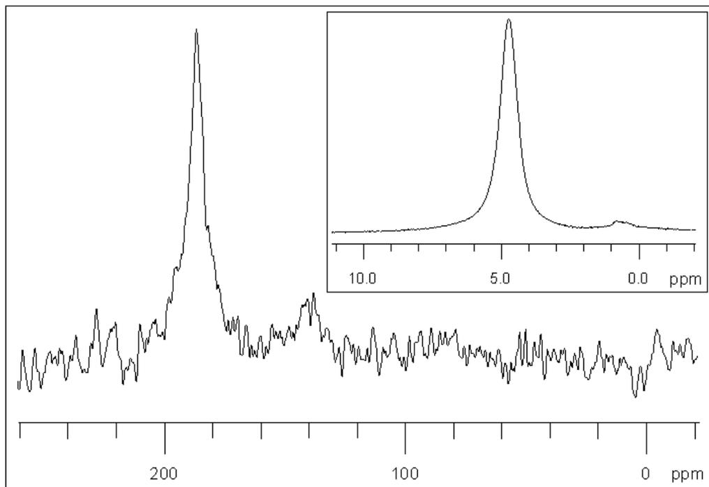
**Figure 4.10.:**  $^{13}\text{C}$  MAS spectrum of a powder sample obtained from the rostrum of the Tendaguru belemnite (*Belemnopsis* sp.) with the project-internal number 9. Inset: Corresponding  $^1\text{H}$  MAS spectrum. Both spectra were obtained at a spinning frequency of 10 kHz and calibrated against TMS in a separate experiment under otherwise identical conditions.
