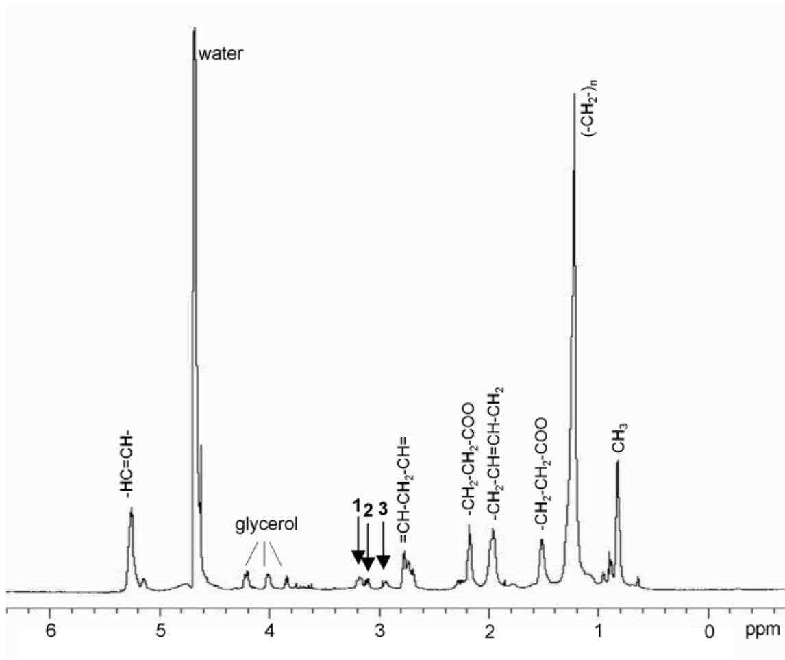
**Figure 2.7.:**  $^1\text{H}$  MAS MR spectrum of *Xenopus laevis* oocytes. Four oocytes were spun at 2.8 kHz. Arrows indicate phospholipids (28). 1: phosphatidylcholine, 2: choline, 3: creatine. Water peak is referenced to 4.7 ppm.
