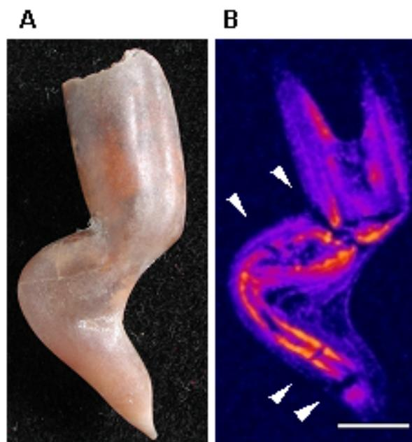
**Figure 4.3.:** Sublethal injury with fracture of the rostrum. *Goniot euthis quadrata* (Blainville, 1827) guard with a zigzag-like deformation. (A): lateral view (photomicrograph). (B): median MR section. Arrow heads indicate fractures. The corresponding slice series (in steps of 125  $\mu\text{m}$ ) with this orientation is given in Movie 4.3 (M). Acquisition parameters: FOV: 15×15×32 mm<sup>3</sup>, MTX: 128×128×256 pxl<sup>3</sup>, NA: 2, T<sub>exp</sub>: 18 h.
