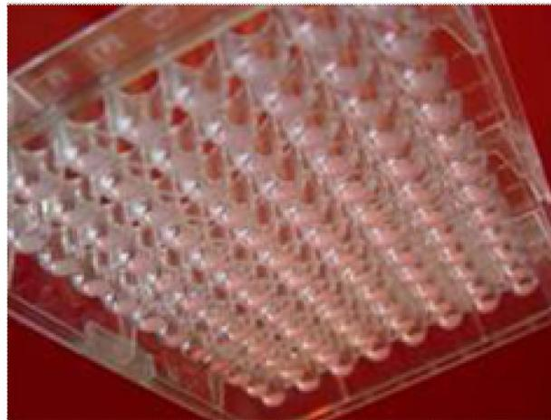
**Figure 4-4** OxoPlate F96, 96-well round bottom microtiter plate with an immobilized oxygen sensor.
