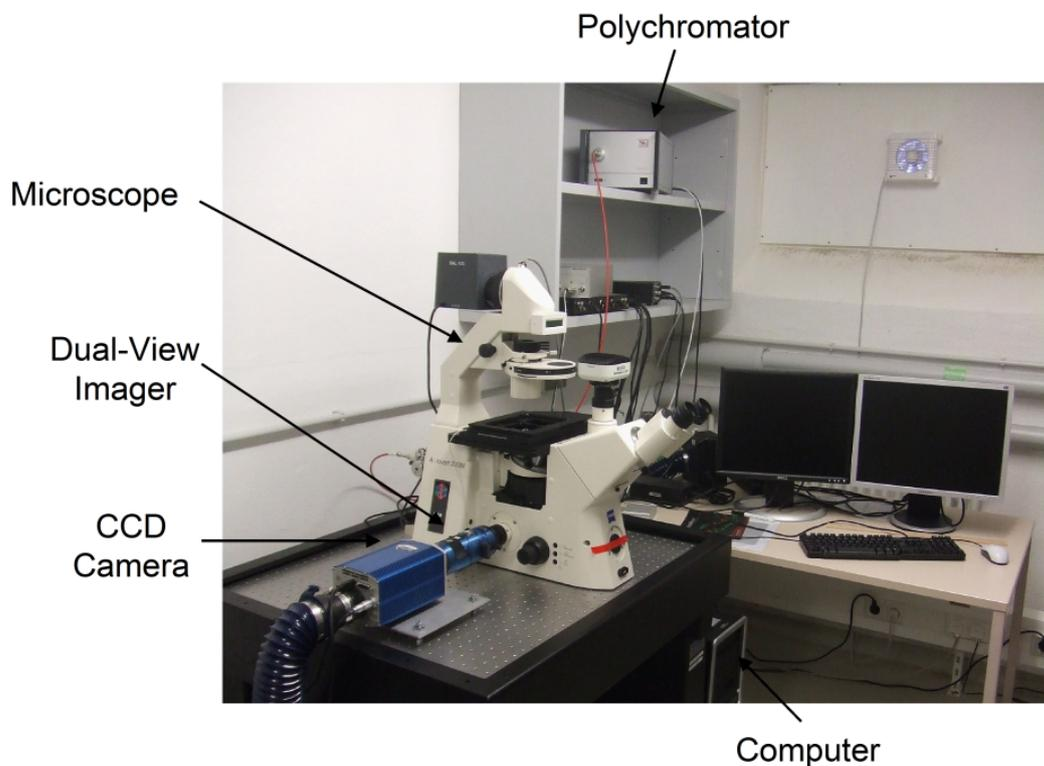
**Figure 2.7: Calcium imaging microscope**
