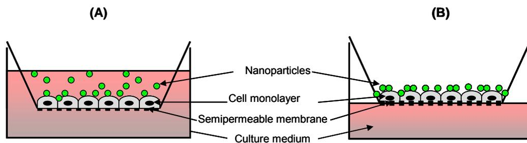
**Figure 1:** Schematic presentation of nanoparticle deposition on (A) Liquid-liquid culture, and (B) AIC
