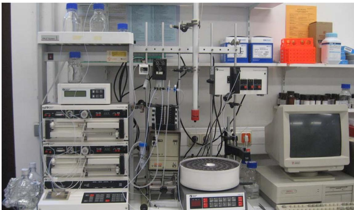
**Figure 2: FPLC for large scale purification of nanoparticles**
