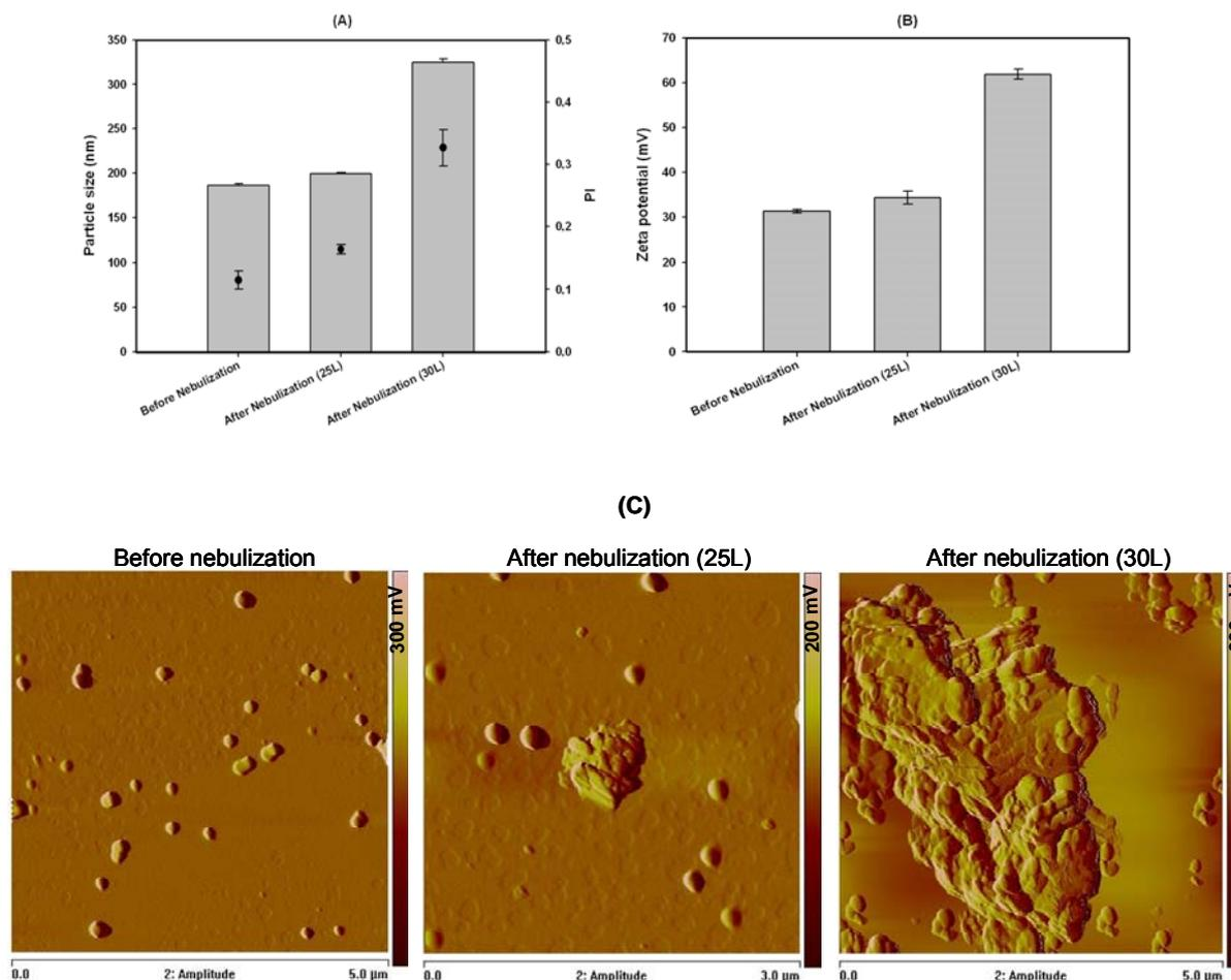
**Figure 3:** Nebulization of nanoparticles using the electronic mesh nebulizer eFlow<sup>®</sup> (A) particle size and size distribution, (B)  $\zeta$ -potential and (C) particle morphology as observed by SPM.
