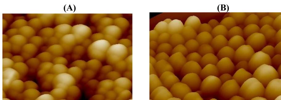
**Figure 1: Morphology of non-modified (A) and chitosan-modified (B) PLGA nanoparticles as observed by the SPM**
