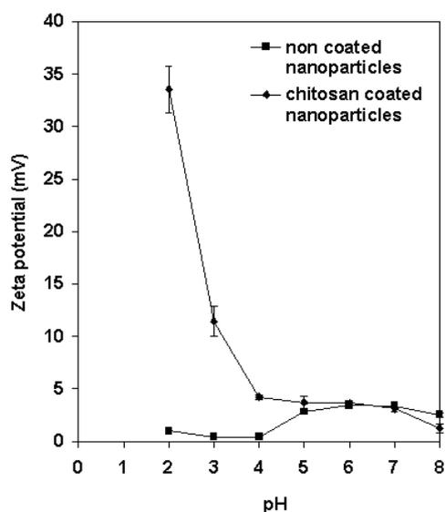
**Figure 2:  $\zeta$ -potential – pH profile for non-modified and chitosan-modified PLGA nanoparticles**
