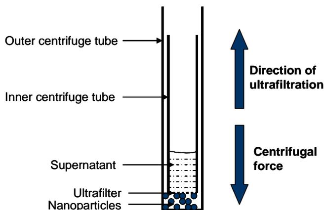
**Figure 1:** Schematic presentation of Centrisart I® and the forces acting during the separation procedure
