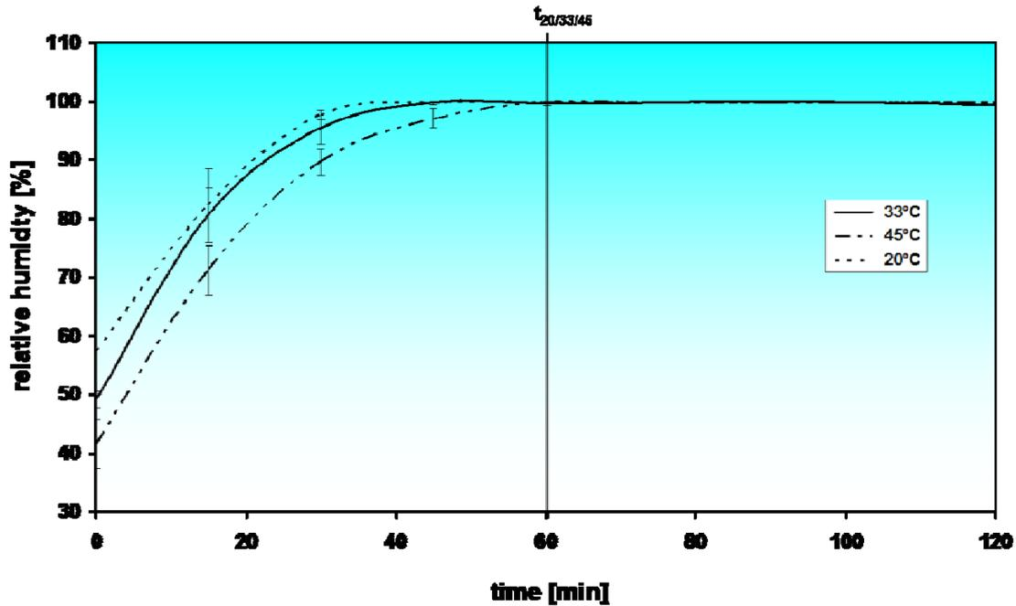
**Figure 12: Experimental Set-up: Course of Humidity**
