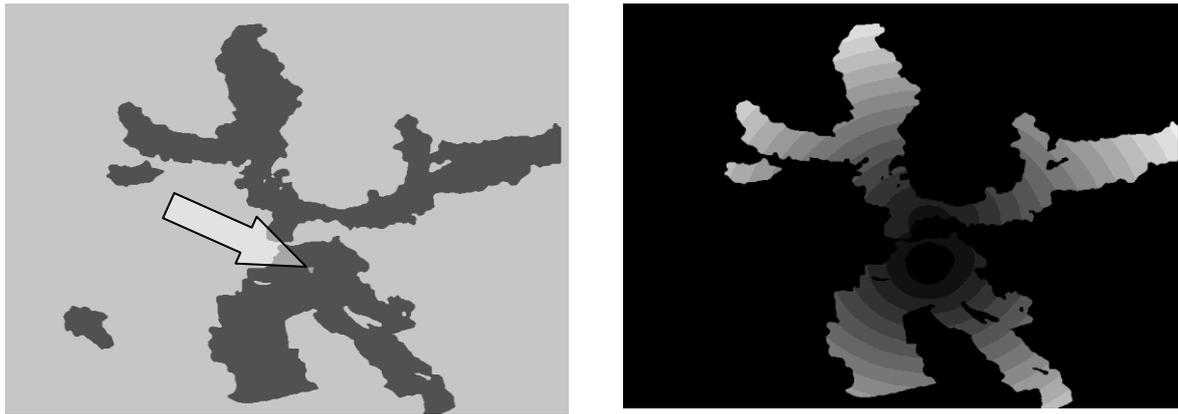
Figure 7.22 Demonstration of the Euclidean distance transformation (EDT) on one 2D section (CG1). Each voxel obtains a gray value, which is proportional to its distance from the nucleus. The lighter is the gray value; the further away is the voxel from the nucleus.
