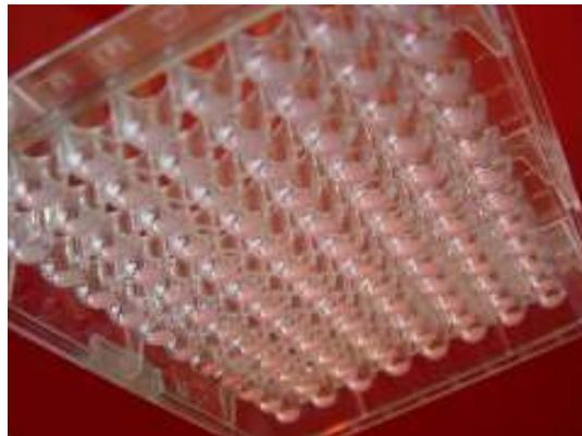
**Figure 4.2.1:** Oxoplate (OP96U) 96 well round bottom MTP with integrated oxygen sensor.
