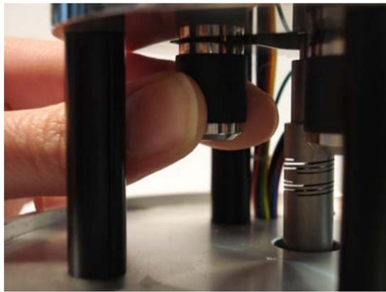
**Figure B.7: Coarse adjustment screws**
