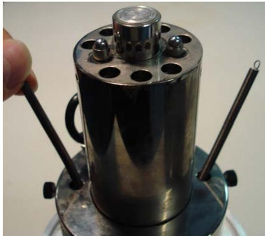
**Figure B.3: Retaining springs**
