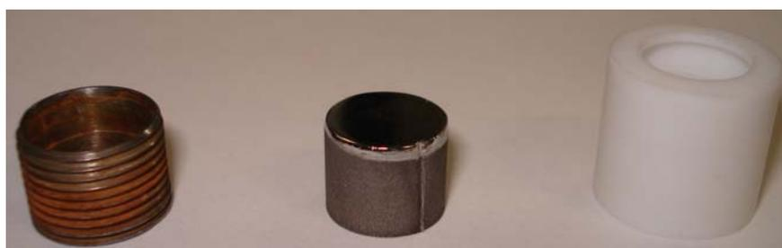
Figure B.2: Electrochemical cell and a typical sample to be fitted into it
