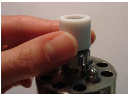
**Figure B.4: Fixing the electrochemical cell on the microscope stage**
