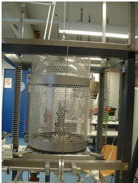
**Figure 4.7: Experimental setup for in situ electrochemical nanoindentation. Protective atmosphere chamber and vibration control.**
