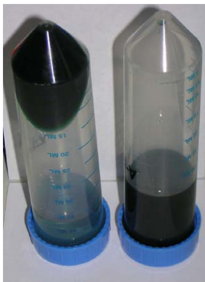
Fig. 40 Dissolution behaviors for composite particles (left) and polyaniline particles (right) into formic acid.
