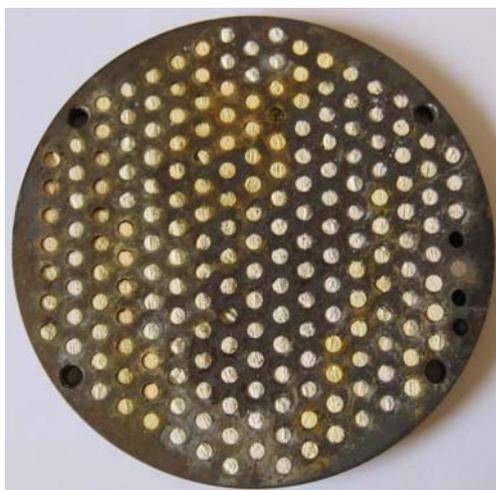
Figure 9. Image of a stainless-steel library plate ( $\varnothing$  99 mm) with 207 hexagonally positioned wells ( $\varnothing$  3.5 mm), filled with catalysts.
