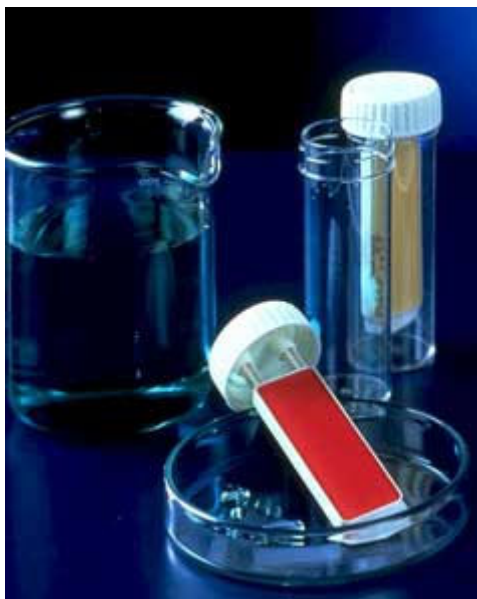
Fig. 2-12. Biotest Hycon Dip Slides: a ready to use system for detection and monitoring of microbial levels in liquids; paddle coated with two different agar media; photograph taken from reference [28]
