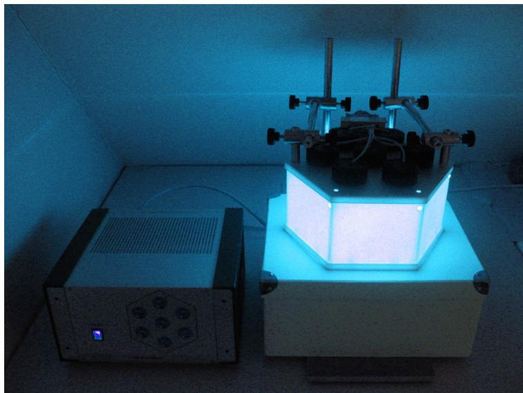
**Figure 5.** Illumination box ( $\lambda = 370$  nm, 2 J/cm<sup>2</sup>)
