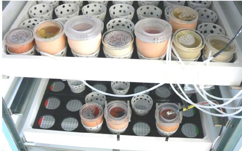
**Figure 5.5: Experimental setup for the thermal measurement of developing chicken embryo with the thermocouple.**
