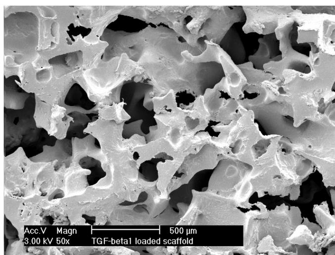
**Fig. 1** Cross sections of a TGF- $\beta$ 1-loaded porous scaffold examined by scanning electron microscopy.
